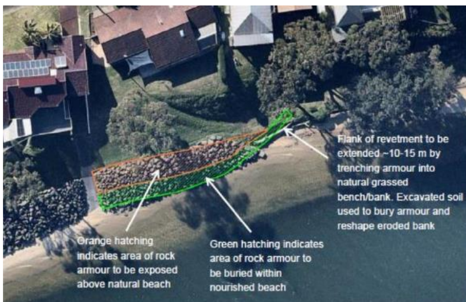
Figure 4. Concept design solution to ameliorate the end effect erosion
